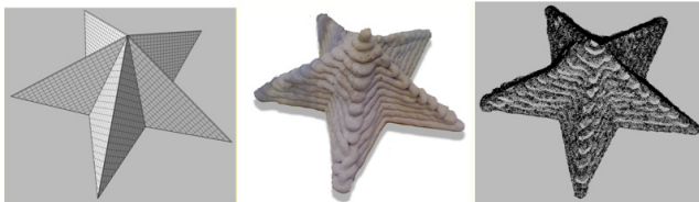
Figure 5: CAD, print and scan model of starfish shape. The filament size of this example is 22 by 15mm to emphasise the error areas.
